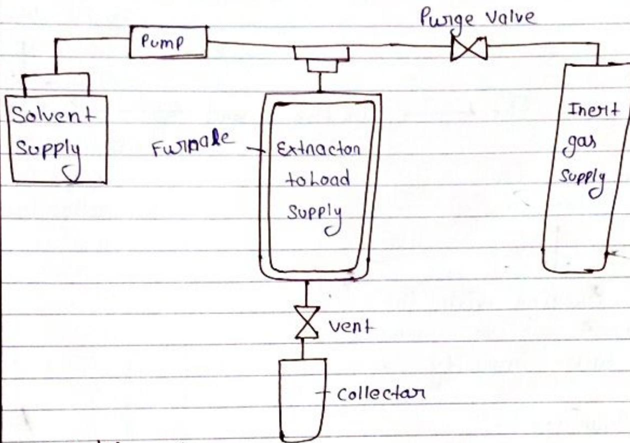
The solvent is filled into the solvent supply chamber and sample is put into the extraction cool temp. maintain to 0 to 100°C & pressure is maintain about 10 to 20 Pascal for some time the extracted material is collected into the collection vial & allow the second solvent to run and collect the extracted material in collection vial by purging it with the inert gas to remove any impurity & to avoid lump formation.
