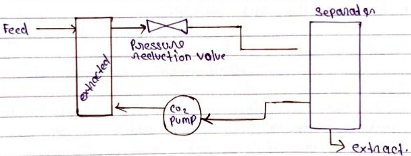
The material to be extracted is feed into the extractor along with the solvent gets in contact with the  $\text{CO}_2$  from  $\text{CO}_2$  pump with high pressure (about 280 pascal) the extracted phytoconstituent is sent to the separator with the low pressure (150-120 pascal) the rough the pressure reduction valve the extracted material is collected w/i the
